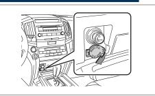
The "ENGINE START STOP" switch must be in ACCESSORY or IGNITION ON mode to be used.
